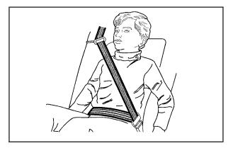
4. Buckle, position, and release the safety belt as described in *Rear Seat Passengers on page 36*. Make sure that the shoulder belt crosses the shoulder.
